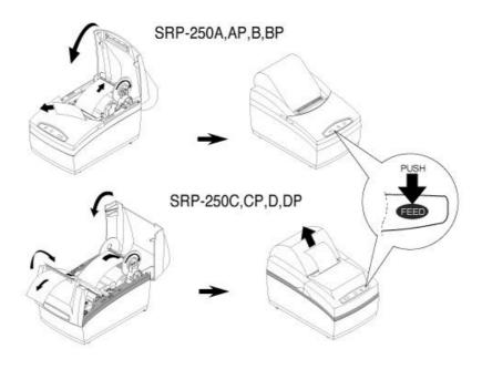
7). Insert the end of the roll paper into the groove on the Roller-Pulley and wrap the paper around the spool two or three times.
